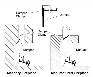
Figure 10 - Attaching Damper Clamp
